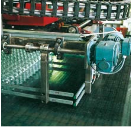
Modules with a smooth surface make accumulating and palletizing bottles on the conveying line possible.
